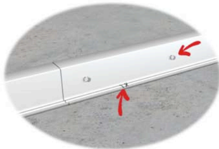
MEASURE & MARK POSITION OF INTERMEDIATE PORTAL FRAMES
