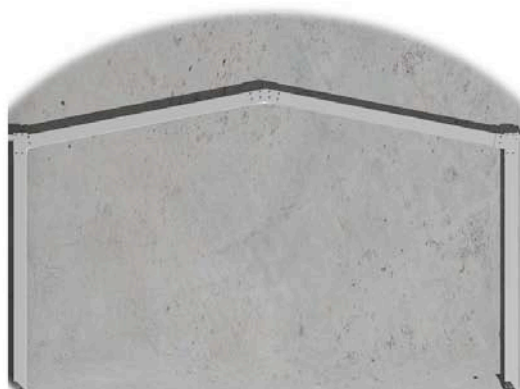
ASSEMBLE PORTAL FRAME ON THE GROUND
