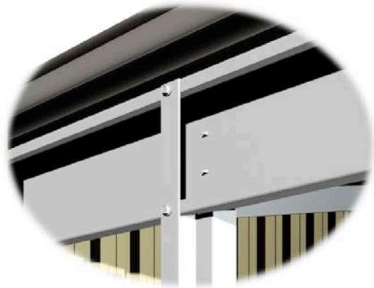
CUT OUT TO FIT OVER RAFTER RAFTER CONNECTION
